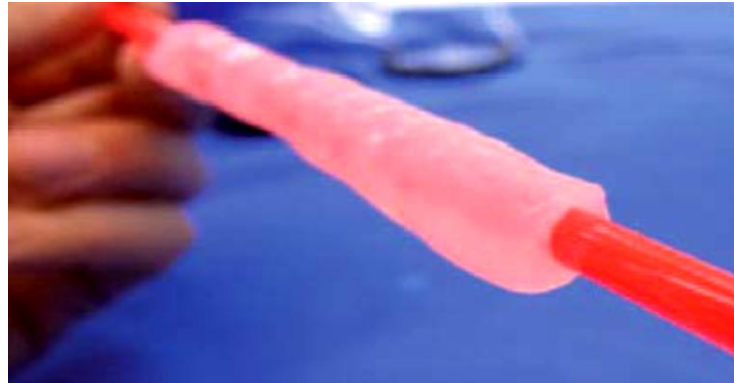
Fig. 6. A tube acting as a blood vessel made of bacterial cellulose, represented on a red glass, symbolizing the blood flow [7]
