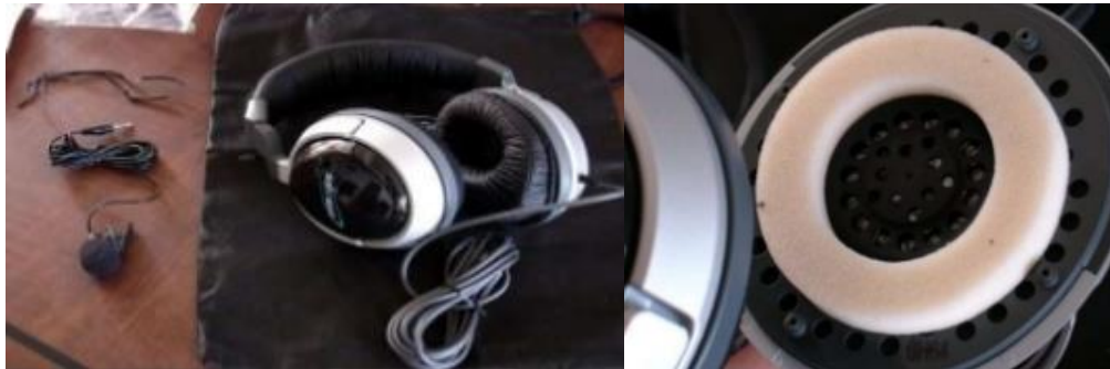
Fig. 12. Biocellulose as membrane transducer in Sony headphones [26]
