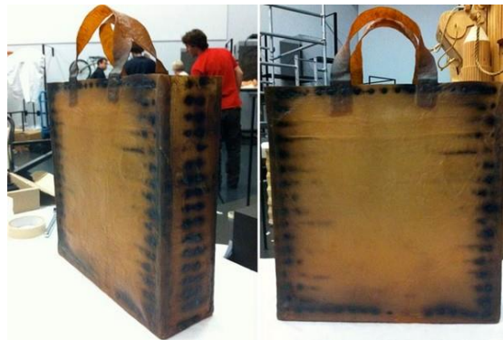
Fig. 11. Biodegradable package obtained from bacterial cellulose [19]
