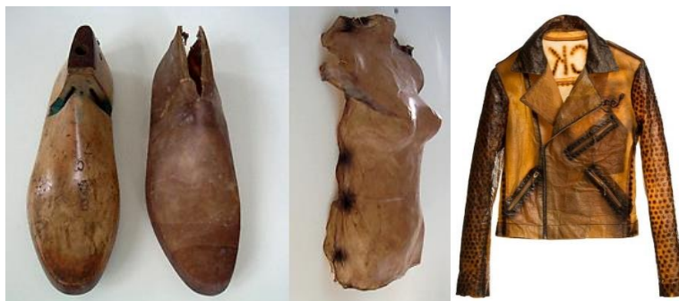
Fig. 9. Clothing and footwear made of bacterial cellulose [16]
