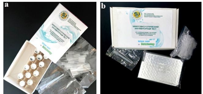
Figure 7 - Prototype microbial inhibitor test based on Bacillus licheniformis T7 spores in microtube (a) and 96-well plate (b) variant
