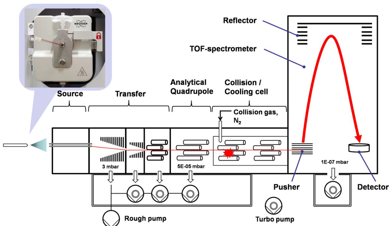
Source (CaptiveSpray, chamber and capillary), ion transfer stage (funnel 1, funnel 2, multipole), quadrupole, collision/cooling cell and TOF spectrometer (orthogonal accelerator (pusher), dual stage reflector, detector)
